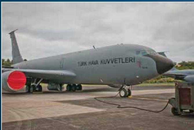
A Lajes Field's Dash 86 power engine belonging to the 65th Operations Support Squadron provides external power to a Turkish air force KC-135 July 19. (Photo by Lucas Silva)
