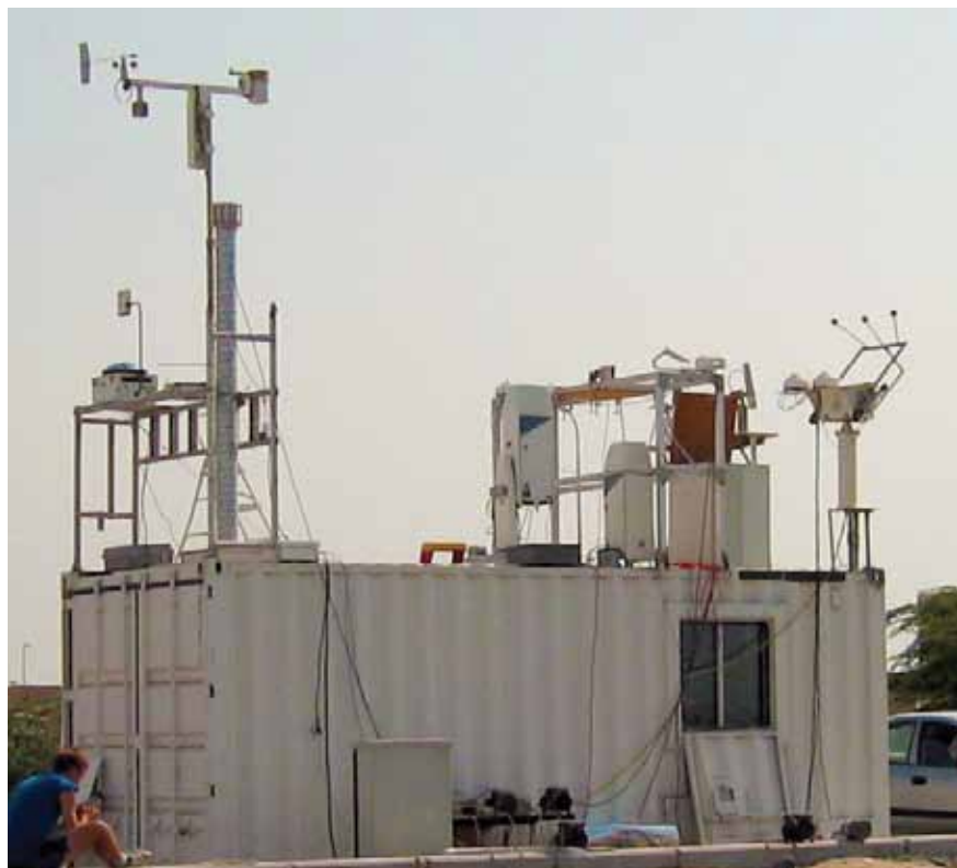
MAARCO is a transportable climate-controlled laboratory containing scientific instrumentation for measuring atmospheric aerosols, trace gases, chemistry, radiative properties, cloud structure, and meteorology.
