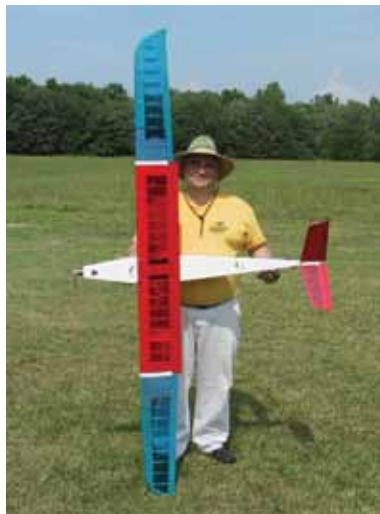
The late James Kellogg, NRL engineer, with the Spider Lion, which flew for 3 hours and 19 minutes on a half-ounce of hydrogen fuel.
