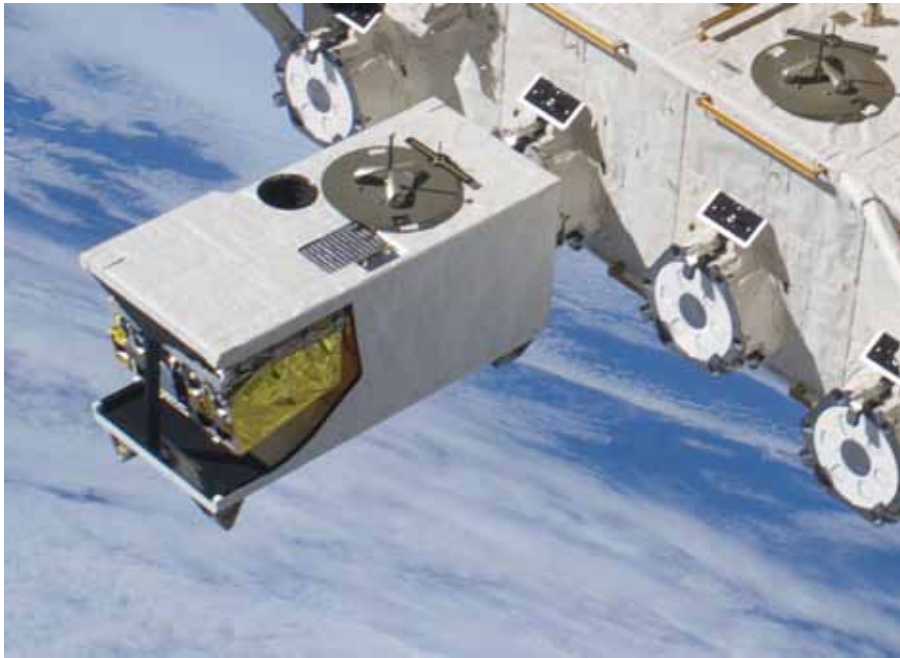
The picture shows HREP's docking position to the JEM-EF. The RAIDS sensor, wrapped in yellow thermal blankets, is pointing to the lower left corner of the picture. The big round feature on the top is the grapple fixture for ISS' maneuverable arm. The black round hole next to this fixture is the baffle for the star tracker. The HICO™ sensor, enclosed by the HREP structure, is located to the right of RAIDS.
