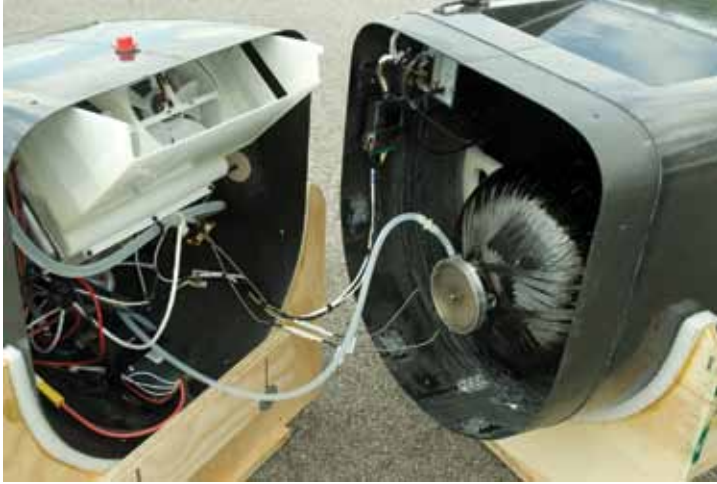
Inside the Ion Tiger: the hydrogen tank and regulator are on the right; the radiator is on the left. The fuel cell is underneath the radiator.
