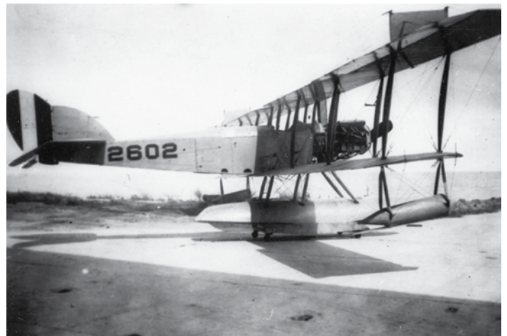
This U.S. Navy Curtiss N-9H floatplane was used in the first radio-controlled flight experiments at Dahlgren, Virginia, 1924.
