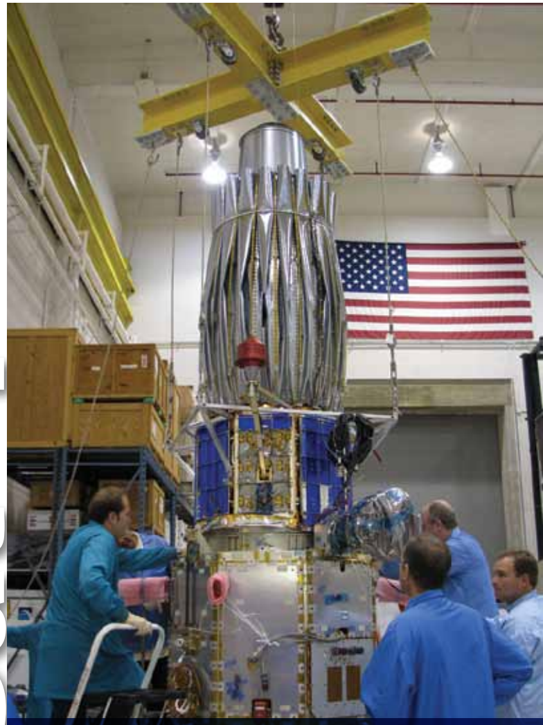
TacSat-4's "COMMx" payload. 12-foot antenna with 10 channels of UHF communications.
