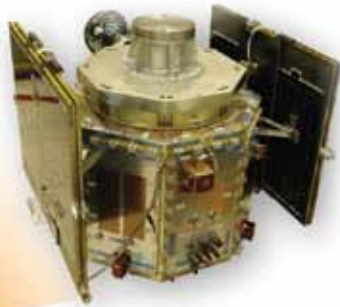
TacSat-4's "COMMx" payload. 12-foot antenna with 10 channels of UHF communications.
