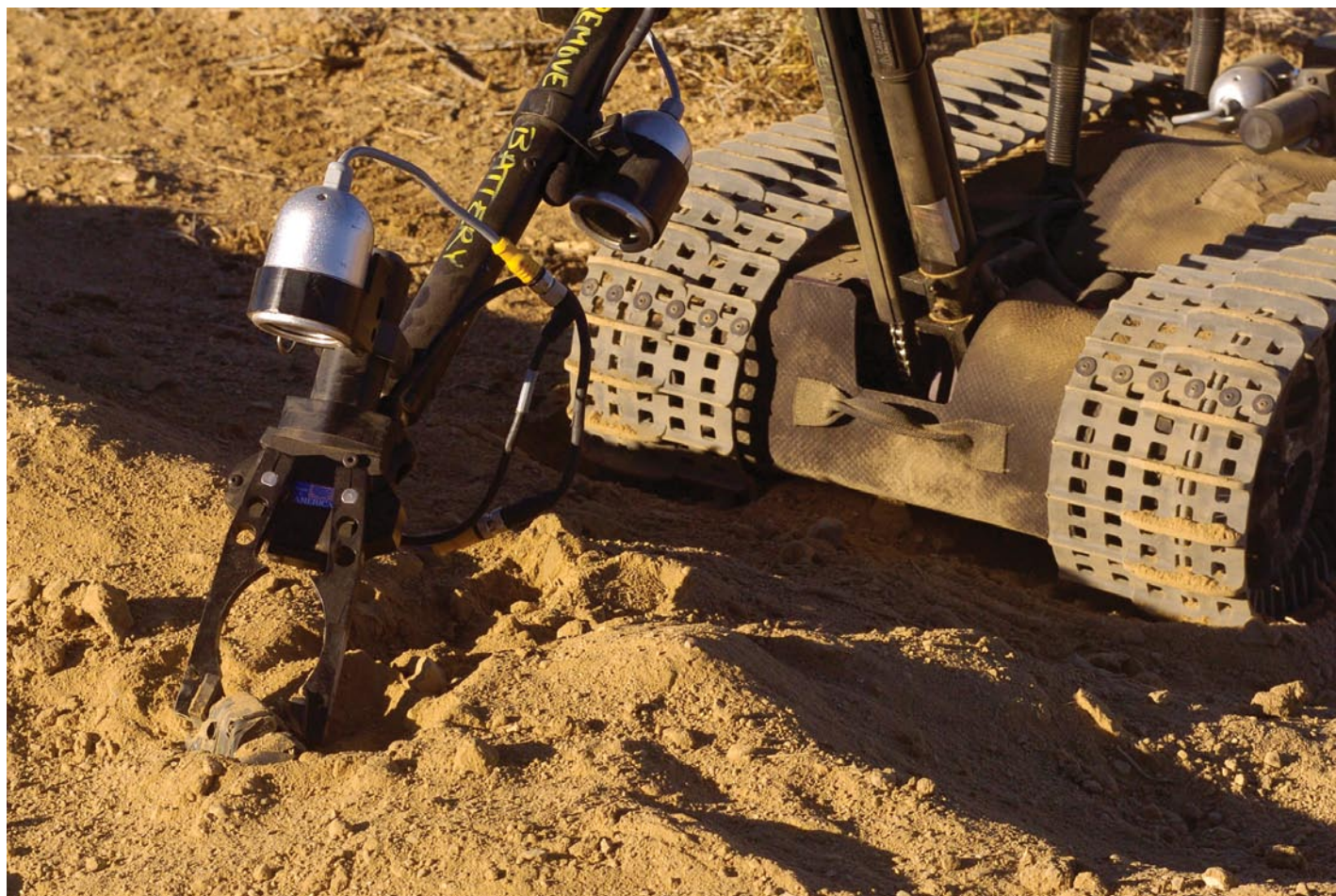
A Talon Mk.II ordnance disposal robot prepares to unearth a simulated improvised explosive device during an exercise.
