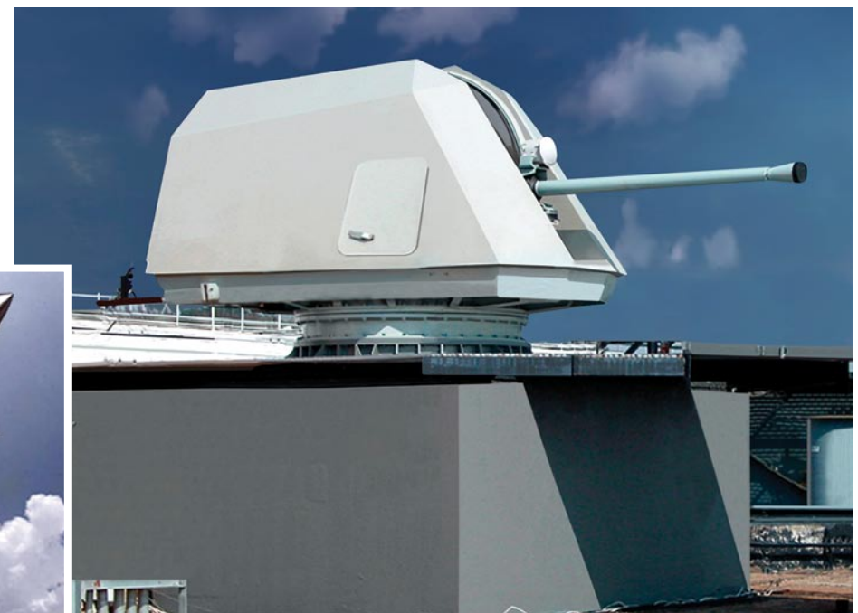
Top The remotely operated MK 38 Mod 2 is a high-speed, highly accurate 25 mm stabilized chain gun that can fire up to 180 rounds per minute to protect ships from attack around the clock in all weather conditions. Above The futuristic Advanced Gun System (AGS) is designed to engage fast-moving enemies in dispersed locations without placing forces ashore. Below The MK 110 Medium Caliber gun offers programmable ammunition and an electrohydraulic stabilization system for extremely accurate shooting, even in high sea-state conditions. Bottom left The rapid-fire Long-Range Land Attack Projectile, to be fired by the AGS, uses an optimized combination of gun-launch and rocket-assisted energy and fires from a fully-automated weapon handling and storage magazine.
