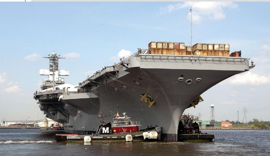
USS George Washington (CVN 73) transits from dry dock to a wet slip. The Norfolk-based Nimitz-class aircraft carrier is undergoing Planned Incremental Availability and Docking. The availability will prepare George Washington to relieve USS Kitty Hawk (CV 63) as the Fleet's forward-deployed carrier in 2008.
