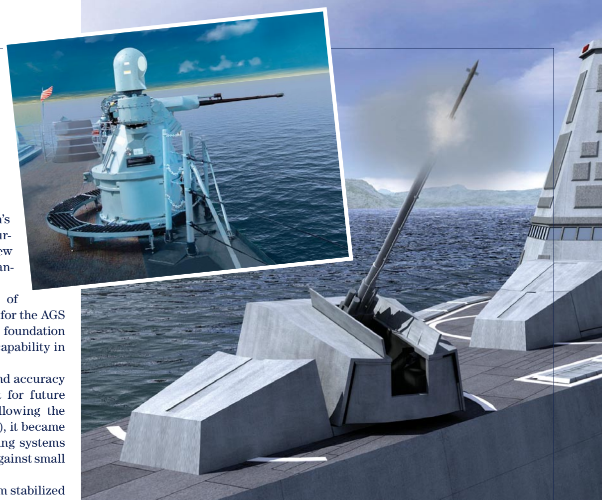
Top The remotely operated MK 38 Mod 2 is a high-speed, highly accurate 25 mm stabilized chain gun that can fire up to 180 rounds per minute to protect ships from attack around the clock in all weather conditions. Above The futuristic Advanced Gun System (AGS) is designed to engage fast-moving enemies in dispersed locations without placing forces ashore. Below The MK 110 Medium Caliber gun offers programmable ammunition and an electrohydraulic stabilization system for extremely accurate shooting, even in high sea-state conditions. Bottom left The rapid-fire Long-Range Land Attack Projectile, to be fired by the AGS, uses an optimized combination of gun-launch and rocket-assisted energy and fires from a fully-automated weapon handling and storage magazine.
