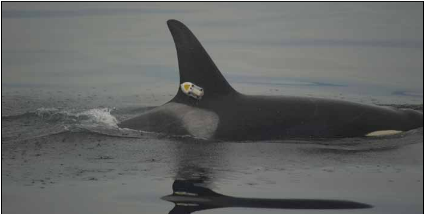
Juvenile killer whale equipped with a digital recording tag. The tag is attached by four suction cups and records the whale's underwater movements as well as any sounds it makes or hears. Photo by Volker Deecke
