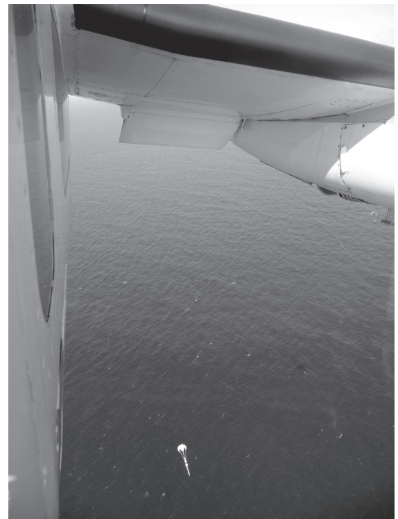
Figure 8. A sonobuoy being dropped from the belly port of the Aerocommander during the 2009 right whale aerial survey. Photo by Jeff Foster.
