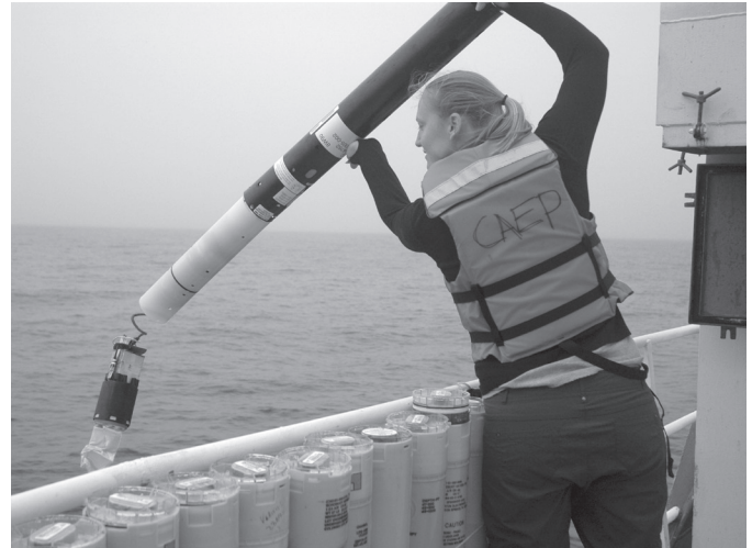
Figure 7. Deploying a sonobuoy from the rail of the NOAA ship Oscar Dyson .
