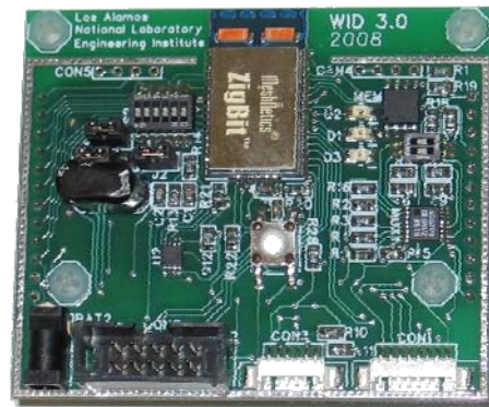
Figure 9: The wireless impedance device (WID3) developed at the Engineering Institute.
