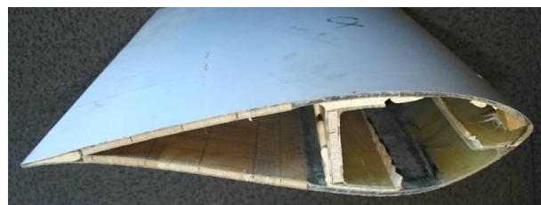
Fig. 1: X-section of the experimental CX-100 blade.
