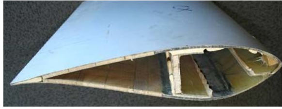
Fig. 1: X-section of the experimental CX-100 blade.
