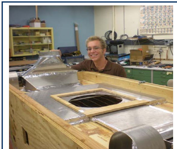
Photo credit: Lisa Hunter, University of Hawaii. James Linden built this thermal enclosure for the ATS telescope.
