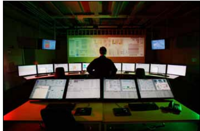
Figure 12.2 HAMMLAB control room simulator
