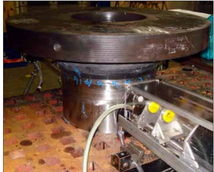
Figure 9.13 Pressurizer surge nozzle DM weld mockup being measured for WRS
