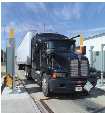
Stationary portal monitors are used to survey the contents of vehicles entering and exiting nuclear power plants.
