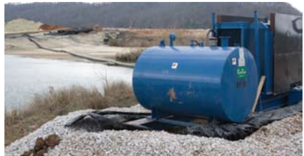
Left: A barge with hydraulic dredging equipment removes ash from the river through the pipe supported by the orange buoys shown here. Top right: Ash and water are pumped through this pipeline. Bottom right: A relay pump operates in the middle of the pipeline.
