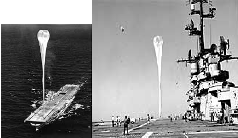
Left: The ten-million cubic foot "Winzen" research balloon on the flight deck of the USS Valley Forge (CVS-45) just prior to launching, during Operation "Skyhook" January 30, 1960. The balloon carried scientific devices to measure and record primary cosmic rays at 18-to-22 miles altitude. Official U.S. Navy Photograph, from the collections of the Naval Historical Center. Right: Tracer balloons are launched from the carrier to test upper atmosphere wind conditions, during Operation "Skyhook". A ten-million cubic foot research balloon is being prepared for flight at the forward end of the flight deck. Official U.S. Navy Photograph, from the collections of the Naval Historical Center.
