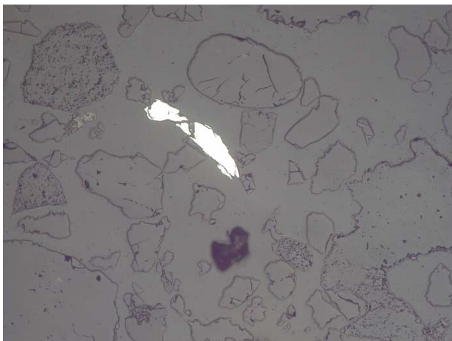
Light Optical Image Figure 10 Scale 1cm = 600 \mu 5575-4 Iron fragment, gangue
