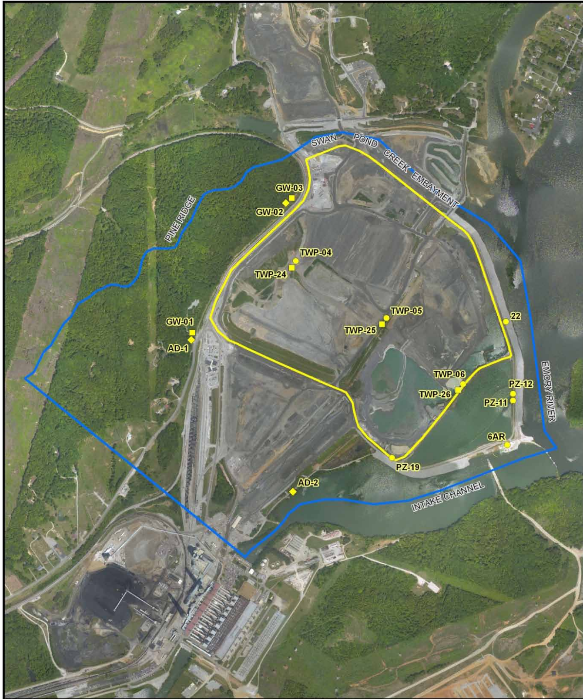
Figure 4-1. Locations of Single-Well Hydraulic Tests and Undisturbed Sampling Locations for Laboratory Analysis of Hydraulic Parameters
