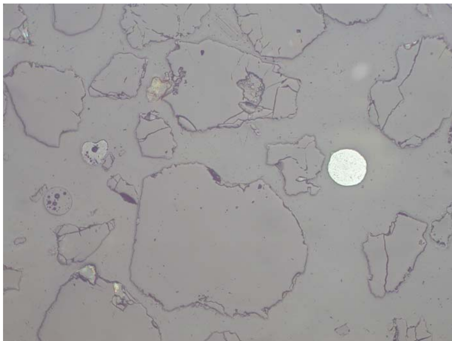
Light Optical Image Figure 7 Scale 1cm = 600 \mu 5575-4 Spherical iron oxide, gangue
