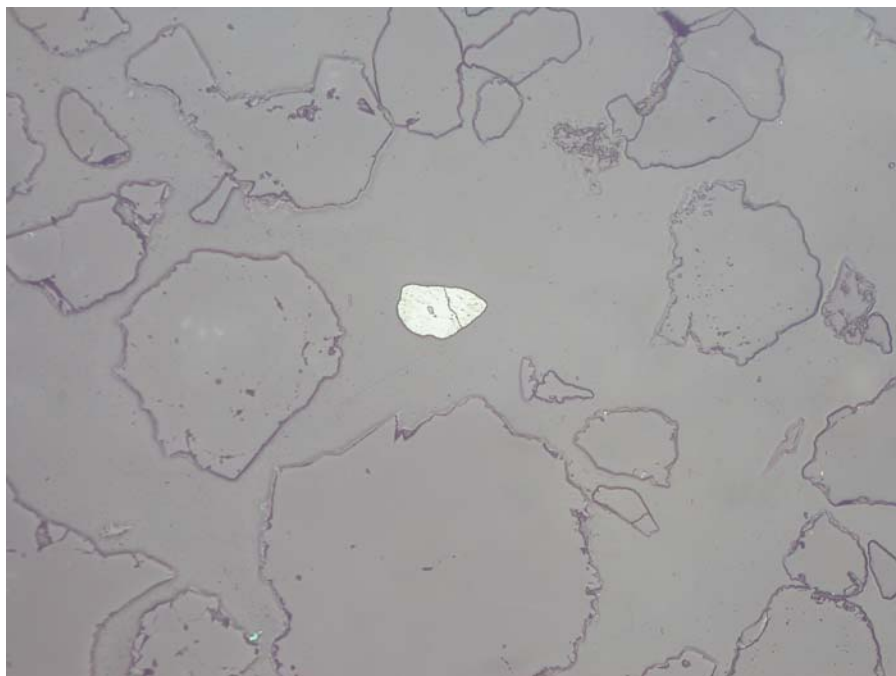
Light Optical Image Figure 15 Scale 1cm = 600 \mu 5575-7 Anatase particle, gangue
