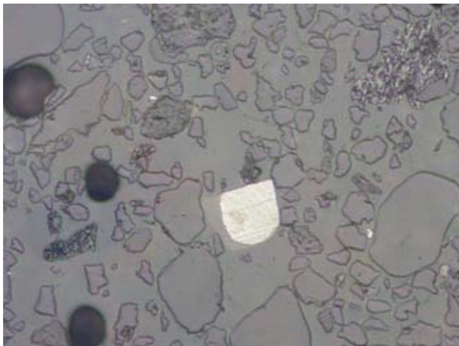
Light Optical Image Figure 9 Scale 1cm = 600 \mu 5575-4 Anatase particle (center), ash sphere (top center), gangue
