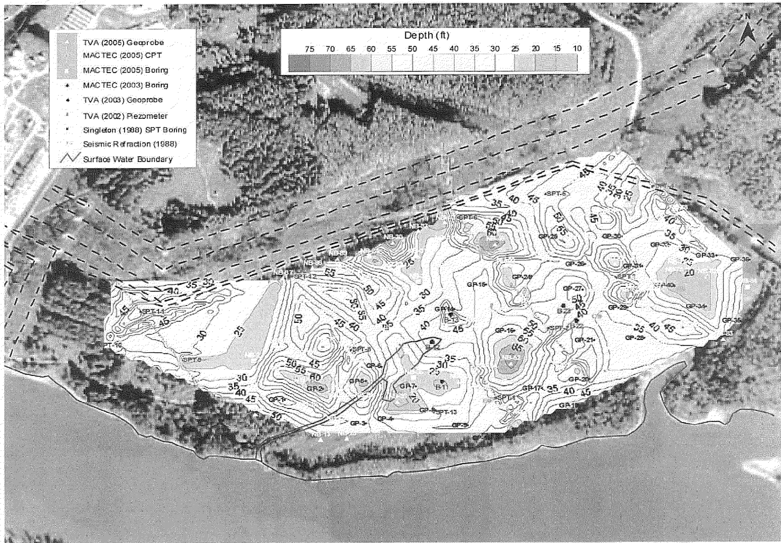
Figure 2-6. Overburden Thickness (ft)
