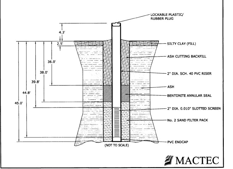
JOB NAME TVA KINGSTON WELL INSTALLATION TVA WELL NUMBER \_\_\_\_\_\_ MW-12 AUGER DIAMETER 3 1/4" (I.D.), 6 1/4" (O.D.) DRILLED BY G. AKINS TOTAL DEPTH \_\_\_\_\_\_\_ 30.0' FIELD REPRESENTATIVE NATE PETERSON
