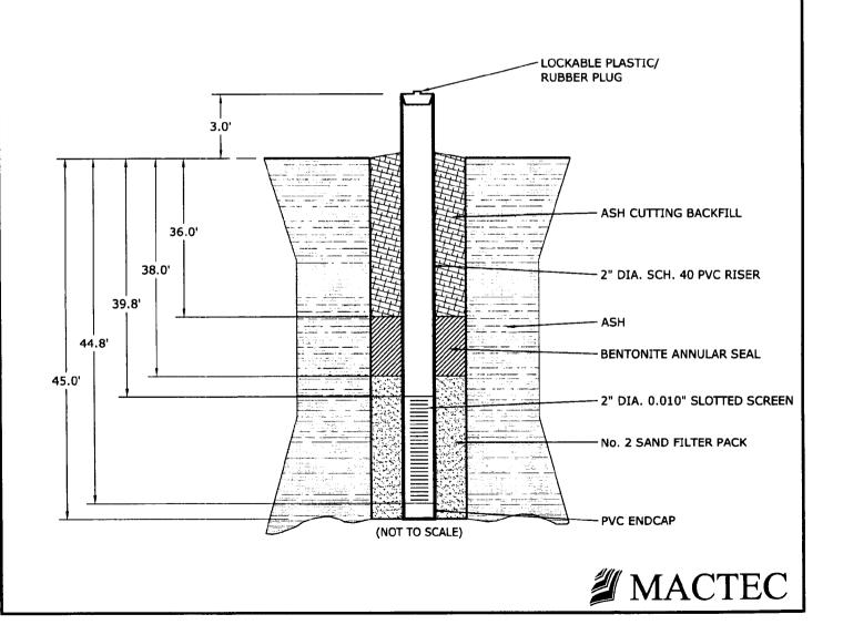
JOB NAME TVA KINGSTON WELL INSTALLATION TVA WELL NUMBER \_\_\_\_\_\_MW-11 AUGER DIAMETER 3 1/4" (I.D.), 6 1/4" (O.D.) DRILLED BY G. AKINS TOTAL DEPTH 45.0' FIELD REPRESENTATIVE \_\_\_\_\_NATE PETERSON
