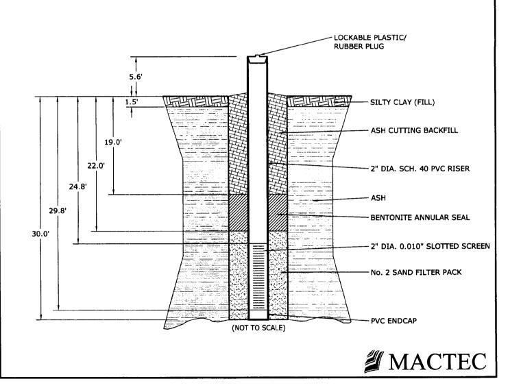
JOB NAME TVA KINGSTON WELL INSTALLATION TVA WELL NUMBER \_\_\_\_\_\_MW-13 AUGER DIAMETER 3 1/4" (I.D.), 6 1/4" (O.D.) DRILLED BY G. AKINS TOTAL DEPTH \_\_\_\_\_\_ 45.0' FIELD REPRESENTATIVE NATE PETERSON
