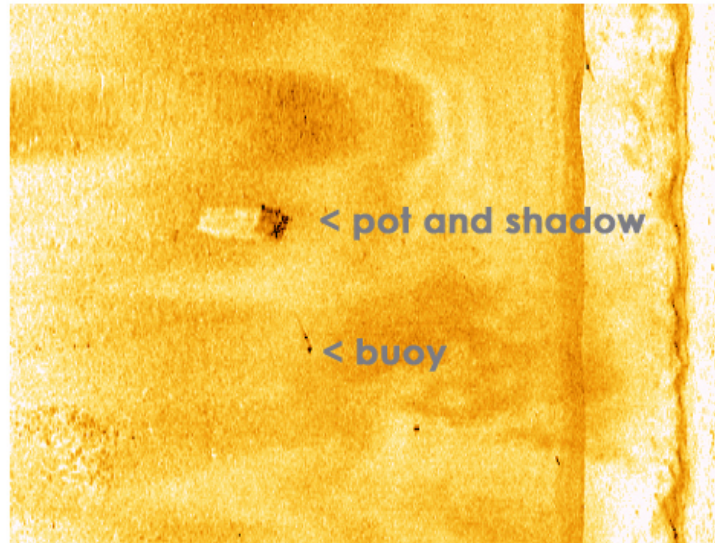
Figure 12. Pot gear with short scope of the buoy line.
