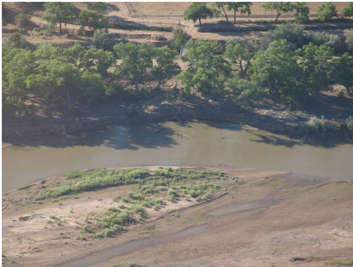
Photo 9: Increased wetted width at higher flows (approximately 1310 cfs) from the Corps of Engineers' bar lowering at the Pueblo of Santa Ana, looking at the RM 205.8 priority site (June 2011, Benoit)
