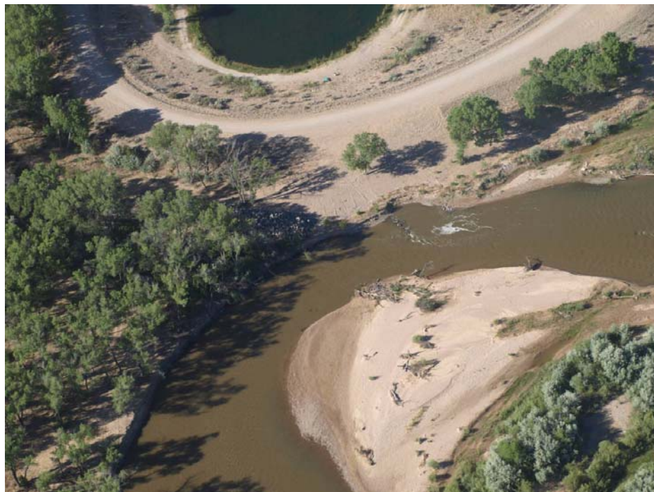
Photo 5: San Ildefonso bankline erosion, riprap windrow, and exposed rock vanes (June 2011, Benoit)
