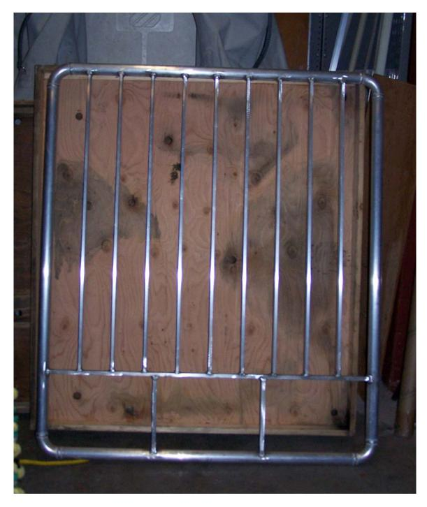
This TED must be fished in the top opening configuration only. Fishing angle of the large frame flounder TED may not exceed 55 degrees from the horizontal. This TED is 25.6% larger than the TED tested in 2007.
