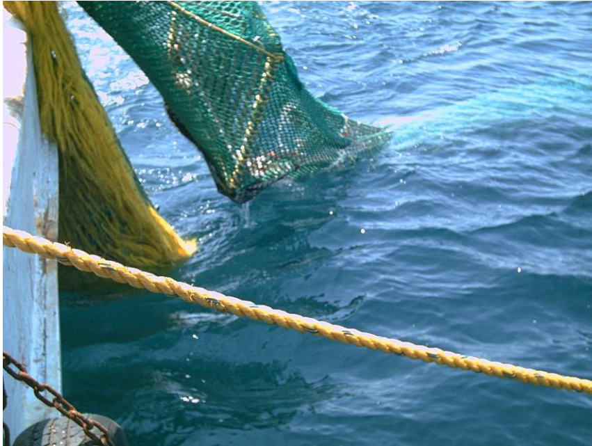
Figure 3. Photograph of accumulated scallops ahead of the TED, that have not moved back into the codend before haulback.
