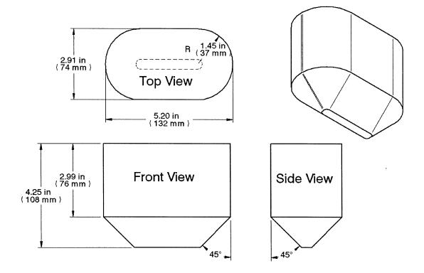
Figure 4: Modified Bath Seat Torso Probe
