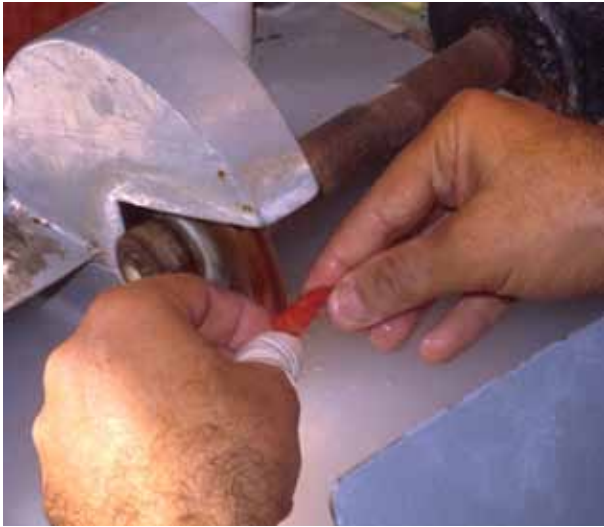
Fig. 1. Cutting coral into bead blanks. The raw coral branches are cut crosswise with an electric diamond-edged circular saw; water is used to cool the saw blade and keep coral dust down. Torre del Greco, May 2000, S.J. Torntore.
