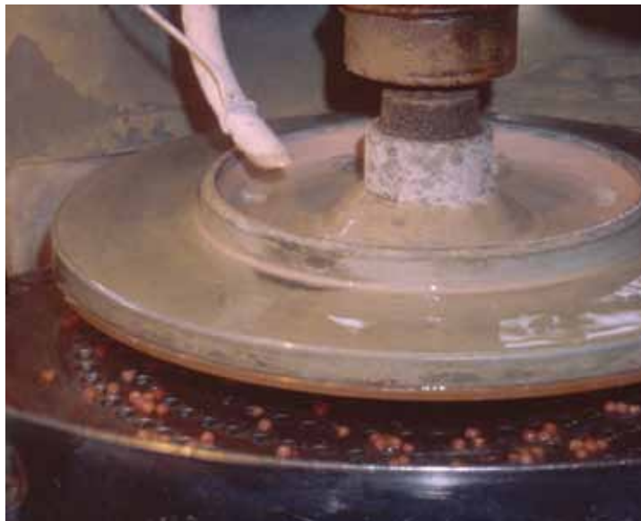
Fig. 4. Making small, spherical pallini beads by machine. Torre del Greco, May 2000, S.J. Torntore.
