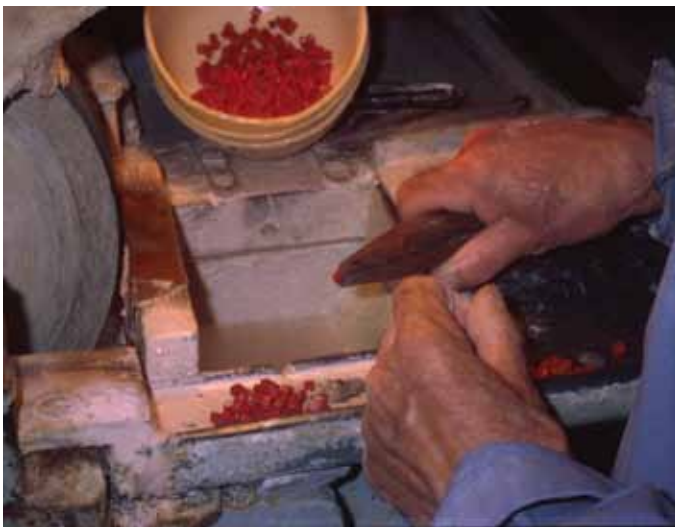
Fig. 3. Rough shaping of the coral bead blanks using an electric carborundum grinding wheel with the coral piece held in a large wooden pliers. Torre del Greco, May 2000, S.J. Torntore.
