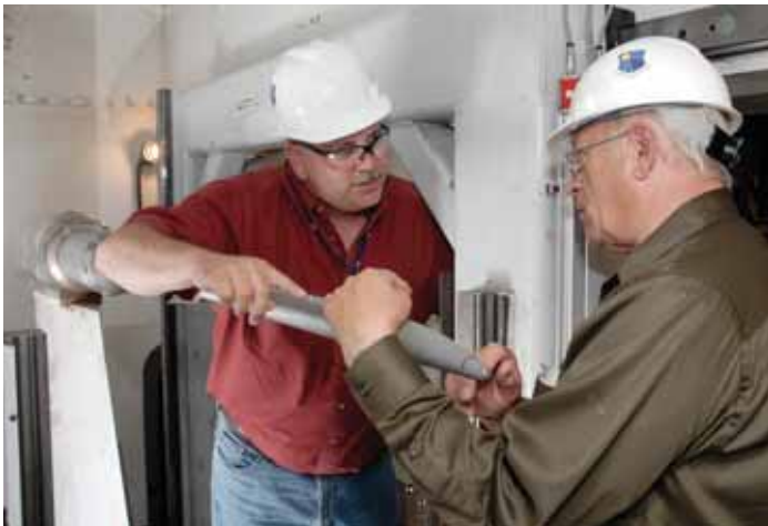
From left, Terry Finley, an engineer with Willbrook Solutions, the Missile Defense Agency support contractor providing aero and test engineering service, and David Carlson, lead test engineer with Raytheon, inspect the Stunner missile model between configuration changes during the testing in Tunnel A.
