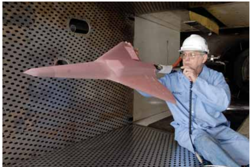
Dennis Odear, ATA outside machinist, inspects a tailless aircraft model in the four-foot transonic wind tunnel while talking to engineers in the control room.
