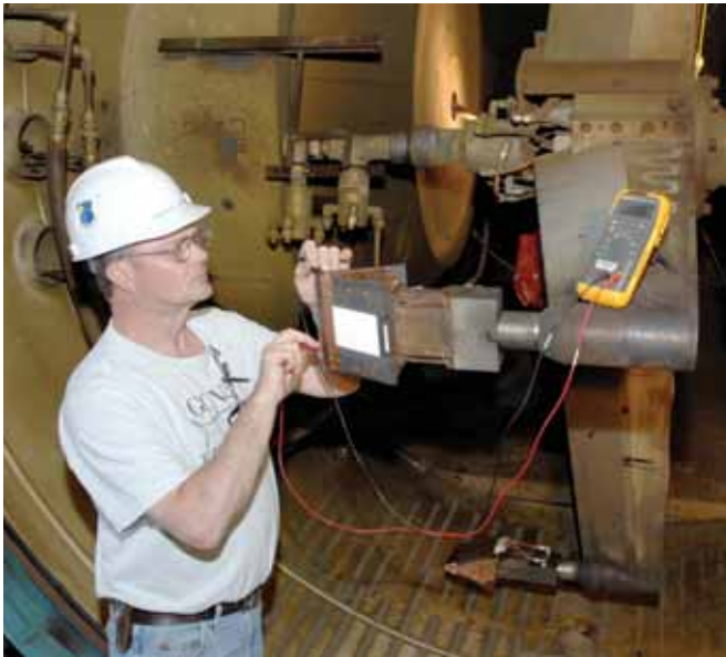
ATA Instrumentation Technician Doyle Jones performs a continuity check on the instrumentation inside the Orion Crew Exploration Vehicle heat shield material candidate model prior to a test run in the H2 test facility.
