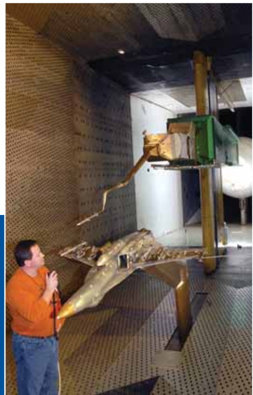
Tim Wright, an ATA outside machinist, coordinates the movement of a 1/10-scale model, sting-mounted AIM-120C store from an F/A-18E/F aircraft during a break in store separation testing inside AEDC's 16-foot transonic wind tunnel.
