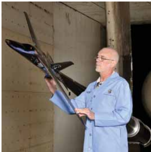
ATA Outside Machinist Carey Wofford inspects the leading edges on the standard check model between tests in 16T.
