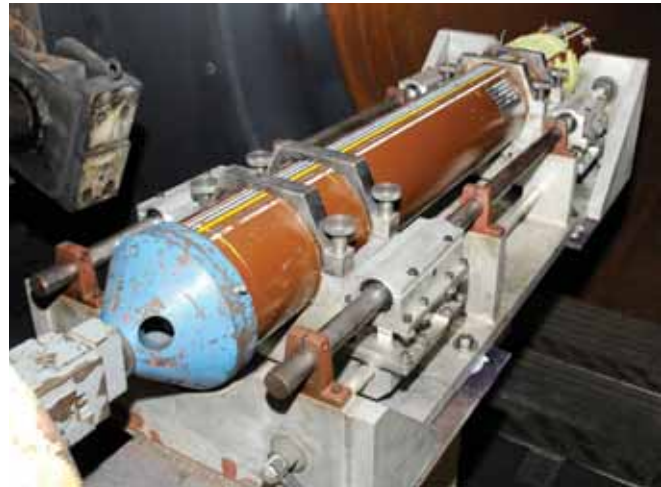
A Multiple Launch Rocket System (MLRS) rocket motor is installed in J-6 Large Rocket Motor Test Facility. Temperature-indicating paint stripes on the top of the MLRS rocket motor monitor temperatures ranging between 200 and 1,200 degrees Fahrenheit.
