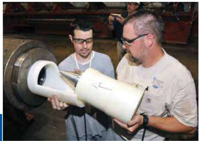
David Brown and Troy Perry, ATA outside machinists, install a slug projectile with a pitch motor installed into the barrel of the Hypervelocity Range G's launcher. This projectile was launched out of the G Range two-stage light gas gun at a velocity of 8,200 feet per second. This was the first test of a new rocket motor that will be used to pitch the Terminal High Altitude Area Defense projectile up to a predetermined angle prior to impacting simulated threat targets. The primary objective of this shot was to verify pitch motor ignition and performance.
