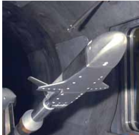
Engineers at AEDC's Tunnel 9 facility performed work on the High-Alpha RLV (left) to examine reentry characteristics. Engineers also performed reentry testing on the Navy's Reentry Systems Nose-tip.
