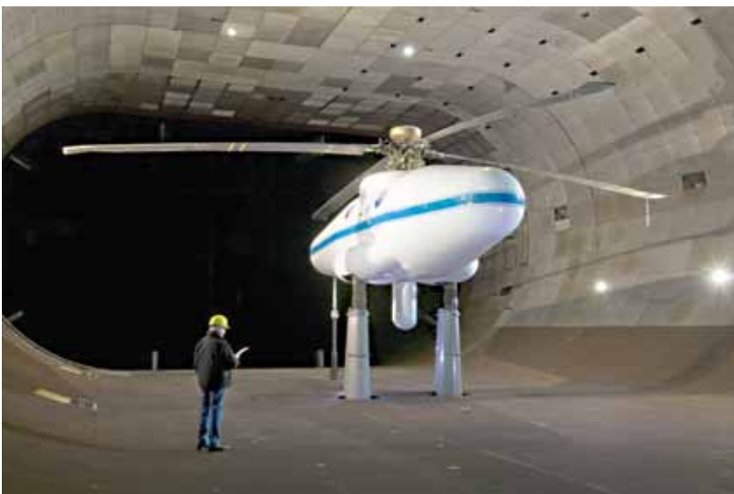
NFAC Test Engineer Al Lizak surveys the large rotor test apparatus test rig prior to testing
