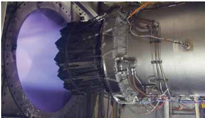
A GE/Rolls-Royce F136 engine, the alternate power plant for the F-35 Lightning II Joint Strike Fighter, is tested at intermediate power conditions. The recent successful altitude testing of the engine took place in the J-2 test cell. The team working on the project was testing augmentor performance and operability to meet mission requirements over a full envelope of altitude and Mach numbers.
