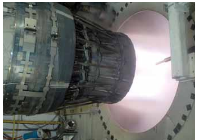
The Pratt & Whitney F100 engine, the power plant for the F-15 Eagle and the F-16 Fighting Falcon, undergoing synthetic fuel testing in the center's J-1 jet engine test cell.
