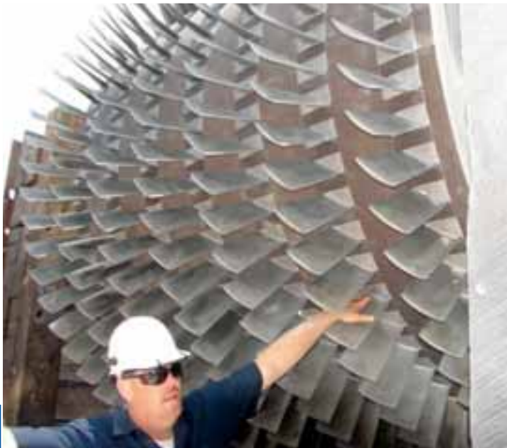
An XS 2 rotor for Engine Test Facility repair.
