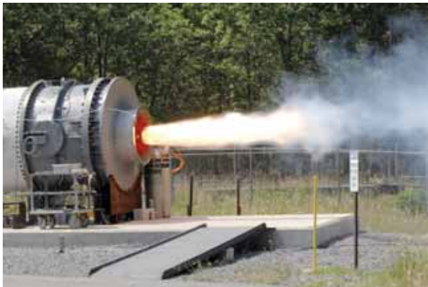
Center engineers ran a series of tests on a Towed Airborne Plume Simulator (TAPS).
