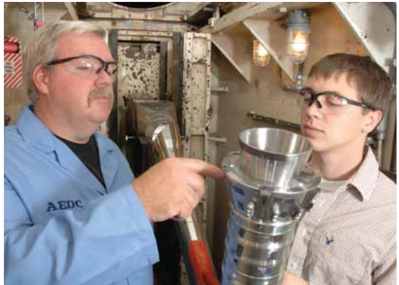
From left, Joe Syler, ATA outside machinist, inspects the Ares I first stage booster model in Tunnel B with Jonathan Kodman, an ATA test engineer.
