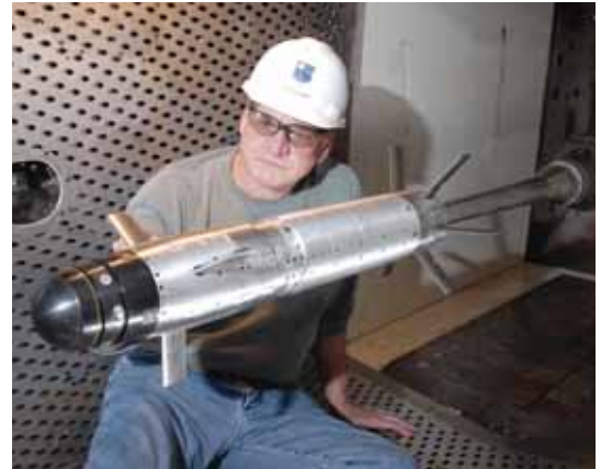
A technician examines the Army's Mid-Range Munition model during aerodynamic testing in the center's four-foot transonic wind tunnel (4T).
