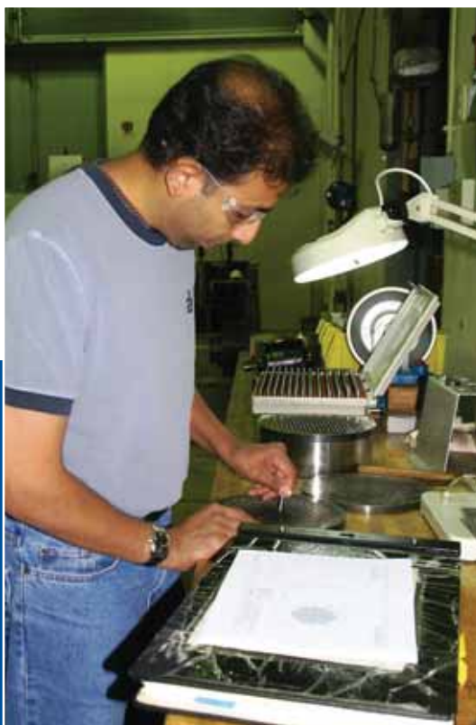
Madhav Rao, an ATA systems engineer at AEDC's Hypervelocity Wind Tunnel 9, inspects one of the holes for ablators that fit into a flow restrictor assembly, which controls flow conditions in the test cell. Ablators, in this case, are devices that lose material from their surface by vaporization and friction during reentry into the Earth's atmosphere. Rao is measuring the holes as part of a redesign effort on the ablator retaining plate, which holds them in place when subjected to simulated reentry conditions during a test.
