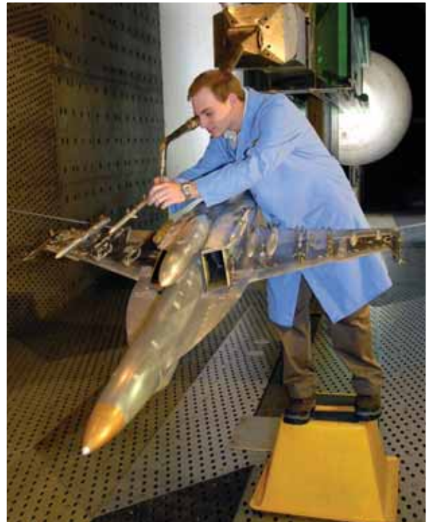
Adam Burt, a co-op student working with ATA, inspects the 1/10-scale models of the sting-mounted AIM-120C store and F/A-18E/F Super Hornet aircraft during a break in store separation testing inside 16T. The testing marked the 13th entry of the Super Hornet for store separation testing in 16T. The data from the testing goes into a database and aids flight testing.
