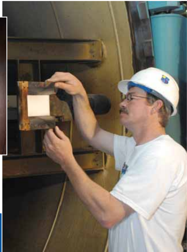
Troy Davis, an ATA outside machinist, checks the alignment of the Orion heat shield material sample prior to testing in H2.
