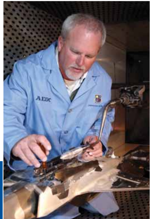
ATA Outside Machinist Jim Lynch makes adjustments to a model of a GBU-31 Joint Direct Attack Munition (JDAM) before a F-35 Lightning II store separation.
