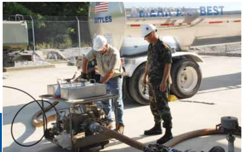
Tech. Sgt. Michael Dambrino, 704th Mission Support Group, Logistics office, watches as Sam McKelvey operates the fuel additive injection rig, which adds chemicals to the synthetic fuel to prevent corrosion and icing, while improving the lubricity of the fuel.
