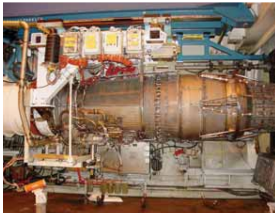
This is a side view of the General Electric F101 engine, the power plant for the B-1B Lancer Bomber, which underwent altitude testing in propulsion J-1 test cell.
