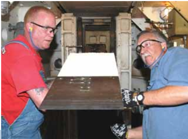
(From left) ATA Outside Machinists Gary Cunningham and R.B. Ray install an External Tank Thermal Protection System foam sample tile prior to injection into Tunnel C which was already running at Mach 4 and 1,440 degrees Fahrenheit. The TPS foam protects the space shuttle's external tank during ascent.
