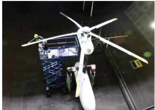
From left, Chris Barkley, a Boeing mechanic, and Oscar Joson, NFAC wind tunnel mechanic, conduct a pre-flight blade inspection on a full-scale, state-of-the-art helicopter rotor system. The test article, a Boeing Corp., SMART helicopter rotor, was tested in the NFAC's 40-by-80-Foot wind tunnel to study the system's forward flight characteristics and to collect data to validate cutting-edge aero-acoustic analysis codes.
