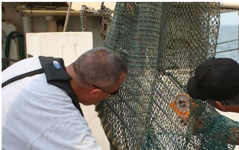
A NOAA special agent and a state partner check the angle of a Turtle Excluder Device. TEDs education and enforcement are a high priority for NOAA's Office of Law Enforcement's Southeast Division.
