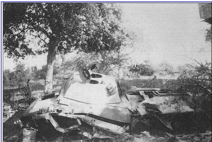
Panzer Lehr vehicles ravaged by the Cobra bombing included this Sd Kfz 234/2 Puma, recon car, mounting a 50-millimeter main battery and a machine gun in the turret. This eight-wheeled vehicle was manned by a crew of four. Robert Hale
