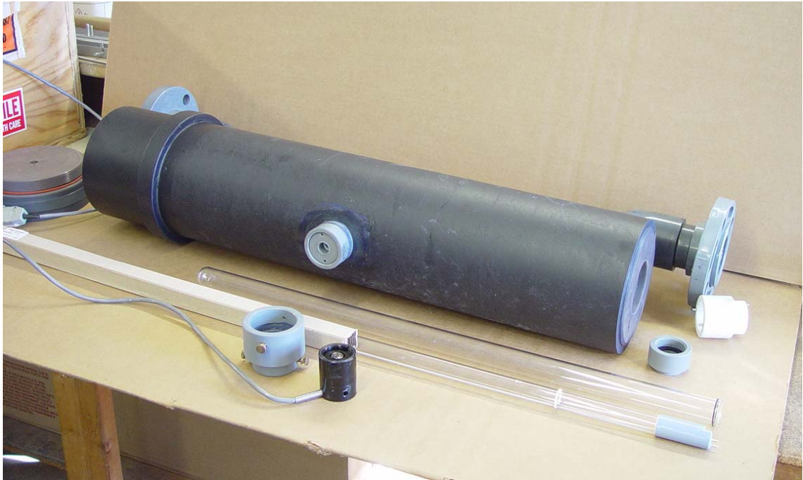
Figure 4: Powerspan's Bench-Scale UV Reactor
