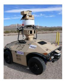
The use of patrol robots to cost effectively improve security while reducing health and safety risks at DOE and NNSA nuclear facilities is an HSS advanced technology deployment "first".
