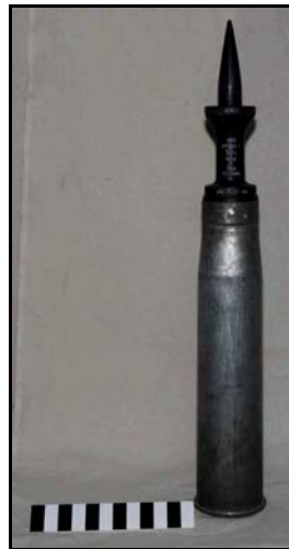
Figure 7-2. DVC-T 17-105 105mm M920 armor-piercing fin-stabilized discarding sabot (APFSDS)
