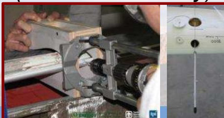
5-Hole Pitot Tube (AOA and Velocity)
