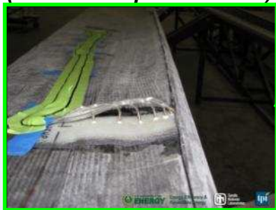
Aero Sensors Pressure Taps (surface pressure)
