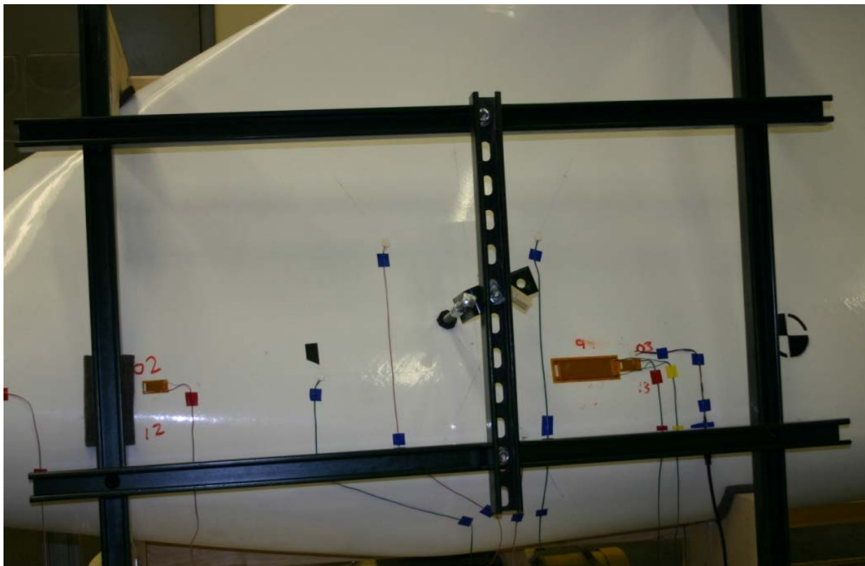
Load Frame used to Apply a Point Load to the Blade
