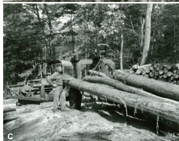
Figure 24.—Horse logging (A) was not uncommon on the BEF up through the 1950s. It was gradually replaced by (B) crawler tractors and finally by (C) rubber-tired skidders. U.S. Forest Service, Northern Research Station, Durham, NH.
