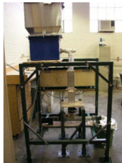
Laboratory-scale of the on-line carbon-in-ash monitor.
