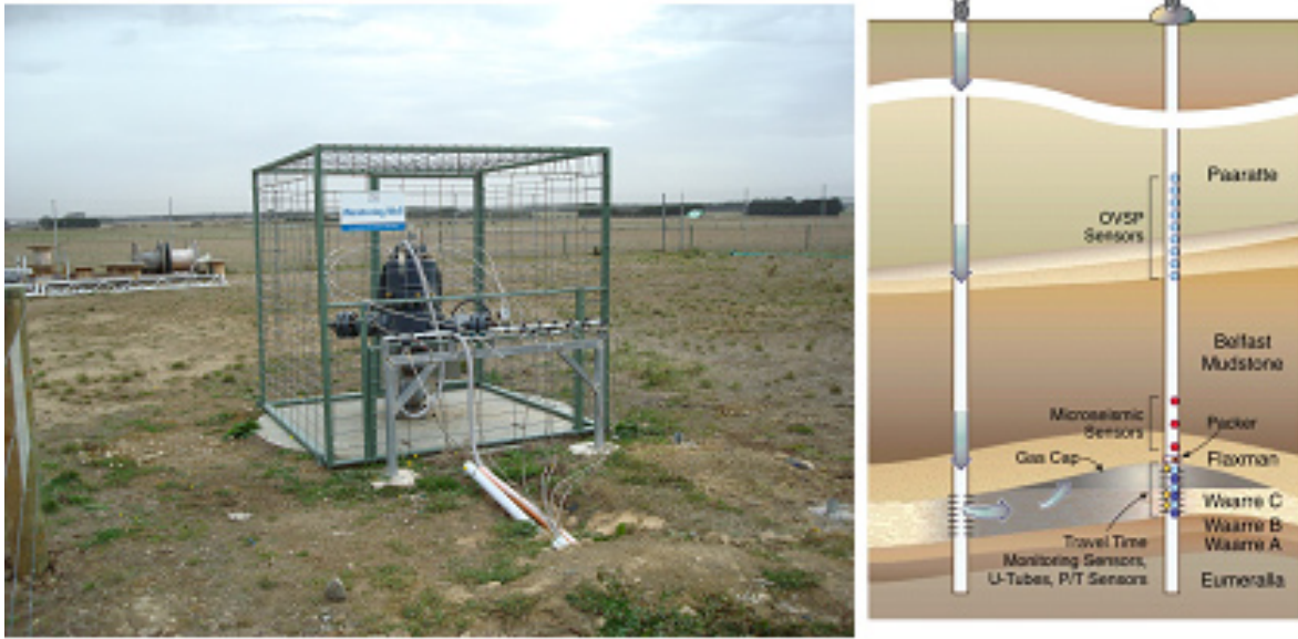
Figure 1: Australian Otway Basin CO 2 Project. Naylor-1 monitoring well (left) and schematic of pilot injection operations (right).
