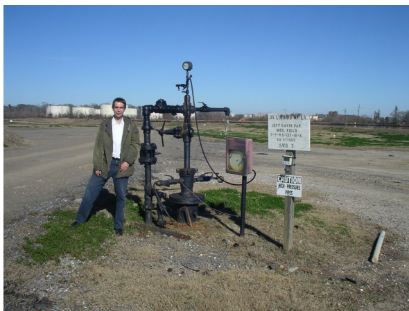
Figure 1: Typical CO 2 injection well at an oil field site.
