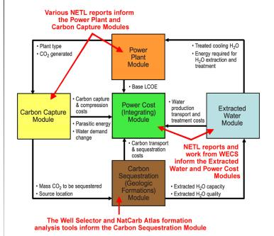
Modular structure of the WECS II model, indicating how the different modules are informed and how they interact
