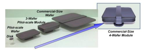
Progression of Reaction Driven ITM Wafer Development – Through material and wafer development, ion transport membranes offer the potential to improve gas separation and reactions for low cost operation. Wafers shown were developed under a separate DOE Cooperative Agreement and enhanced under this project.
