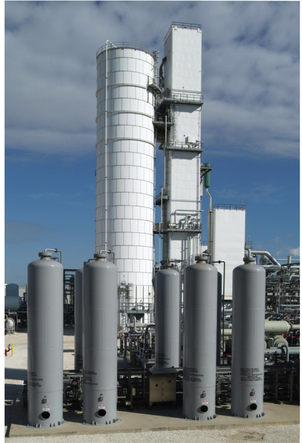
Shown in the foreground is a refinery off-gas PSA at Air Products' facility in Baytown, TX
