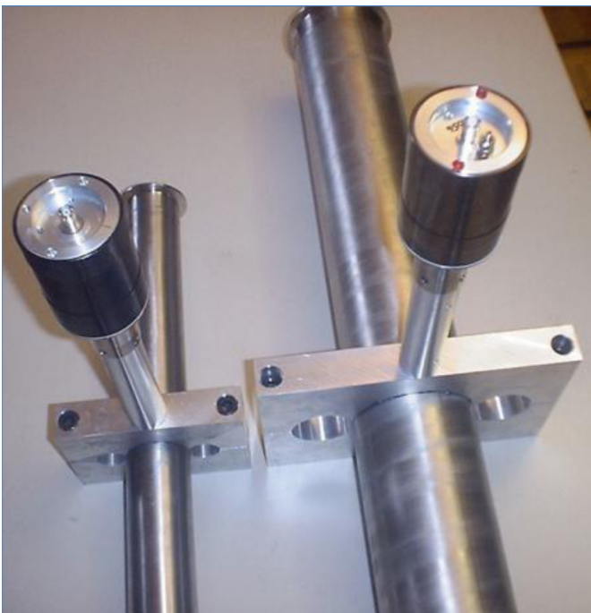
Clamp-on acoustic reactors installed on small and large stainless steel tubing.
