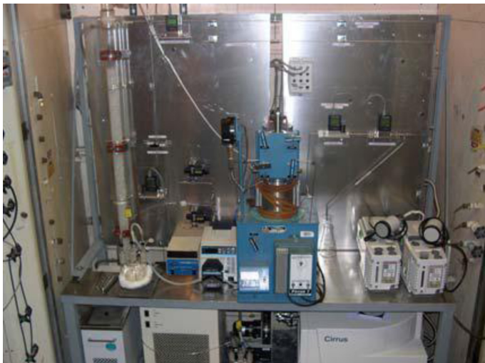
Laboratory-scale continuous CO 2 capture system.
