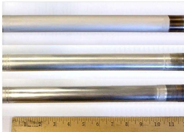
Pre-engineering/pilot scale membranes with membrane area (~ 780 cm 2 ; 1" OD, 10" Long) sufficient to produce > 2 lb H 2 per day
