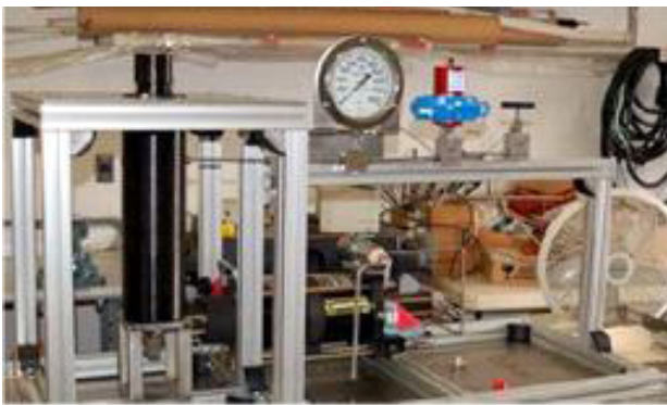
Figure 1: An autoclave is used to create elevated pressures and temperatures. Basalt samples are placed into the autoclave where geochemical analyses can be performed in conditions similar to those encountered within basaltic formations under real world conditions.
