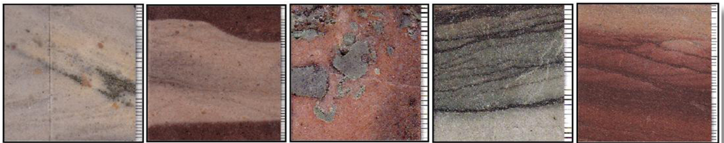
Figure 1. Examples of Mt. Simon Sandstone (a potential CO 2 sink) illustrating its textural and compositional variability.
