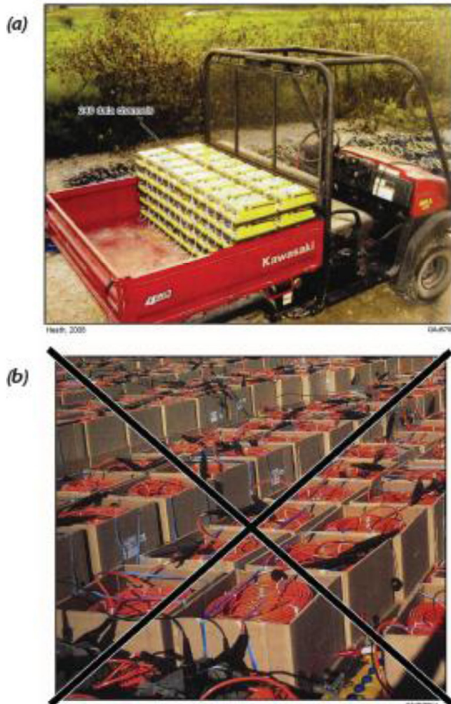
Figure 1a and 1b - (a) Deployment of a 240-channel cable-less data-acquisition system consisting of 80 stations. Several hundred stations will be used in the project under discussion. (b) Just some of the cables that do not have to be deployed in a cable-less operation. In terms of size, weight, manpower demands, and repair costs, seismic spread cables are the major component of conventional cable-based seismic data-acquisition systems.
