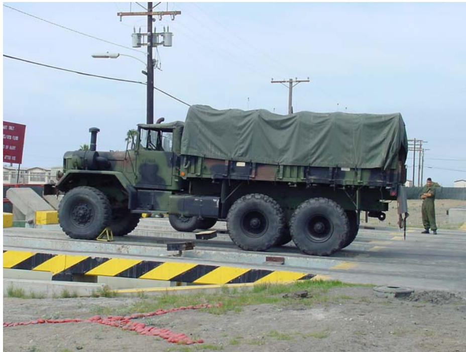
Five-ton on wash rack (note wheels blocked to prevent rolling)
