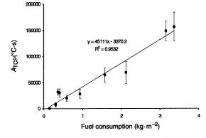
sociated with flame residence time, both at the TCP tip and in the fuel bed. In fact, the ratio of fuel consumption to flame residence time within the fuel bed varied little:  $0.04 \pm 0.01 \text{ kg}\cdot\text{m}^{-2}\cdot\text{s}^{-1}$  (n = 12).
