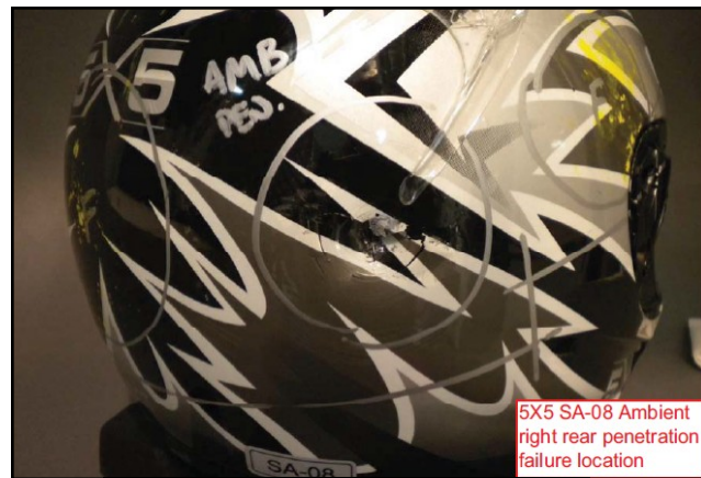
Very easily identified hole in the outer shell of the helmet that classifies this as a fail.
