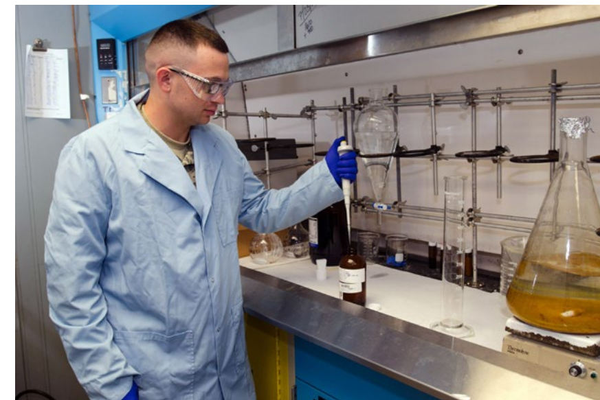
Sgt. Joshua Boudreaux tests the pH of a water sample.
