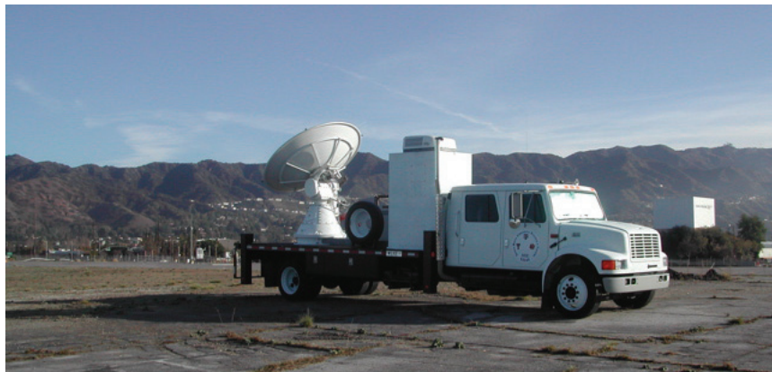
NSSL's SMART-R Doppler C-band radar collected data to help improve debris flow outlooks, watches and warnings.
