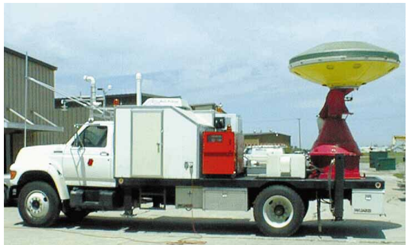
Figure 2: Radars capable of measuring clear air velocity are key mobile sensors proposed for deployment during the TIMEx experiment. The "Doppler-on-Wheels" radar is operated under a cooperative agreement between the JMRF and the National Center for Atmospheric Research (NCAR). Coordinated measurements from two DOW radars that have been deployed near boundaries will permit finely resolved analyses of the evolution and spatial structure of airflow in the planetary boundary layer.
