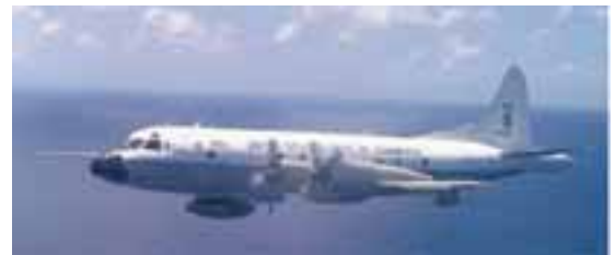
Figure 2: The P-3 (NOAA-42) will make in-situ measurements of pressure, temperature, humidity, and winds (i.e. "state variables"), while also sampling cloud and precipitation content. The helically scanning tail radar alternately points ahead of and behind the aircraft axis, thus providing crossing or "pseudo-dual Doppler" wind and reflectivity measurements as the P-3 flies through the storm.
