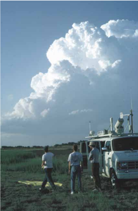
Figure 1: Photograph looking north at newly-developing deep dryline convection at 0040 UTC on 16 May 1991 during the COPS-91 field experiment (courtesy C. Hane, NSSL). The NSSL-2, a mobile ballooning laboratory operated by the Joint Mobile Research Facility (JMRF) of the Oklahoma Weather Center, is in foreground while a developing Wheeler County, Texas storm is in background. Valuable experience gained from COPS and the later VORTEX project on obtaining mobile soundings and other observations both preceding and near developing storms will be applied during TIMEx.
